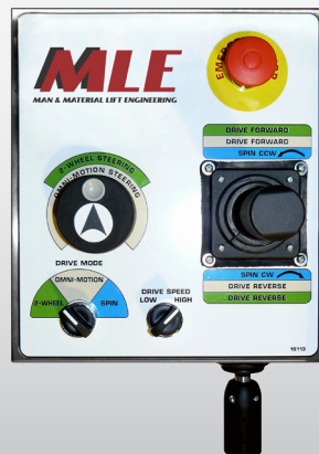
Omni-Motion Drive System Platform Controls
