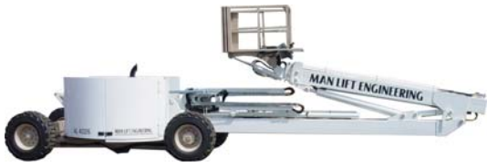
Transport Configuration less than 8-feet high
